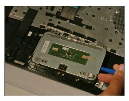
Using the plastic opening tool, lift the touchpad off of the keyboard cover.
