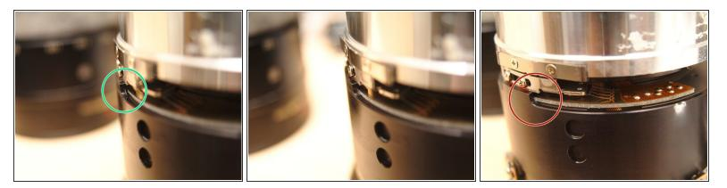
Here is the ISSUE. internal focus ring has contact with Distance readout PCB. The PCB is mounted by double sided tape. This is a design flaw. double sided tape drifts over time, and let the PCB slip out.
