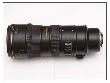
• The lens. Focusing mechanism traps in close-up end, worsens over time.
