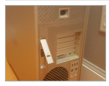
Begin by pulling up on the lever located at the back of the computer to remove the side panel.
