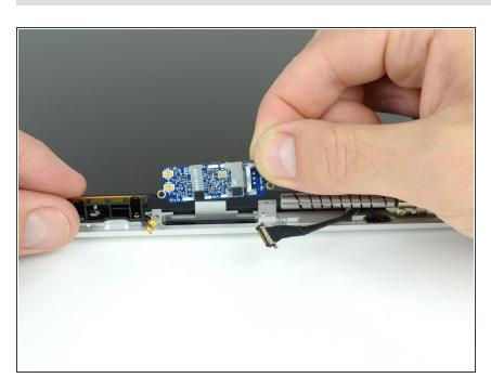
Lift and remove the AirPort board from the display case.
