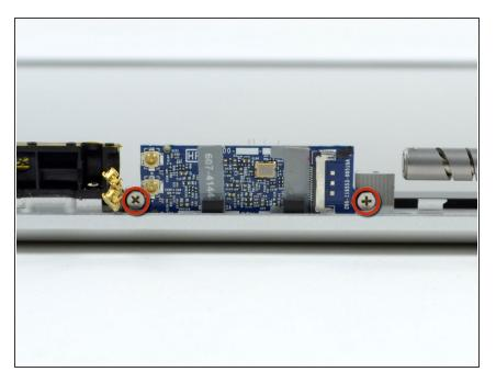
Remove the two 3.1 mm Phillips #00 screws securing the AirPort board to the display case.
