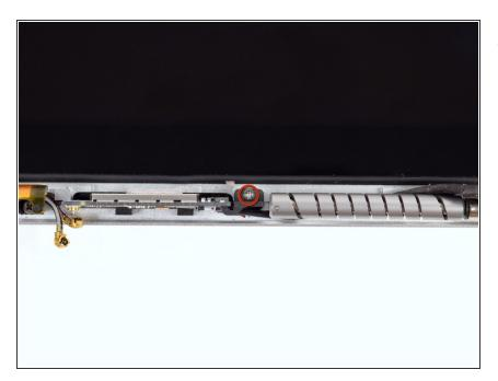
Remove the single 2.7 mm Phillips #00 screw securing the AirPort board bracket to the display case.
