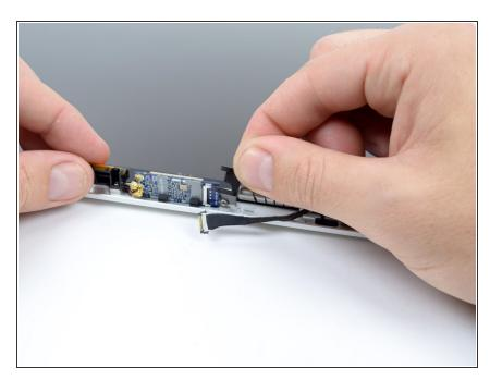
Once the cable is disconnected, lift and remove the plastic bracket from the display case.
