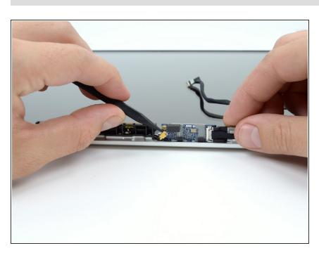
Use the tip of a spudger to disconnect the two antenna cable connectors from the AirPort board.
