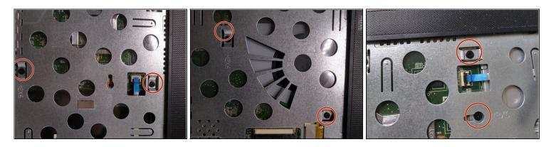
• remove the 6 screws ( m2x6) holding the metal plate to the case.
