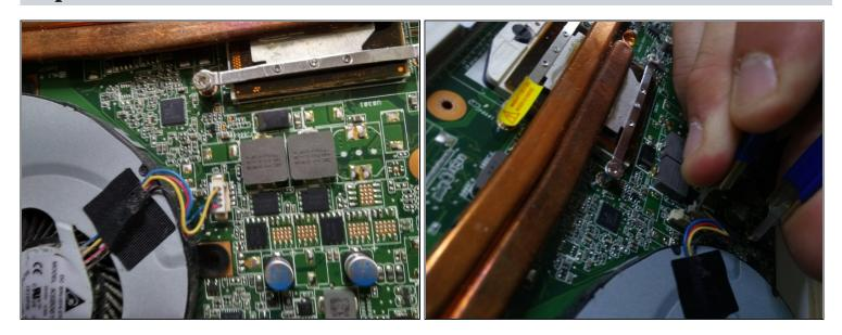
release the fan from the main board by removing the connector with an IC extractor pliers.
