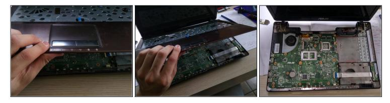
• remove upper plate , revealing the main PCB.
