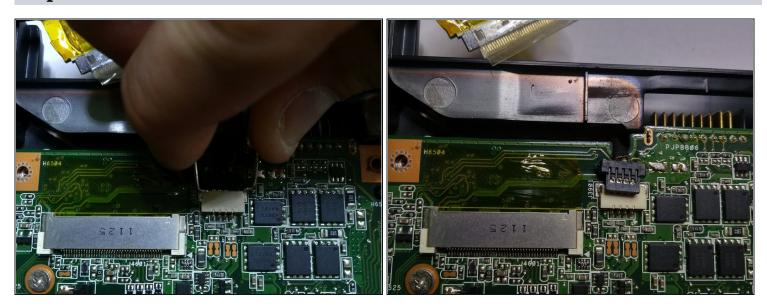
• use IC extractor pliers to remove the cable away from is socket.
