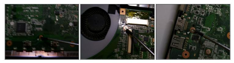
• remove the 4 screws holding the main pcb ..
