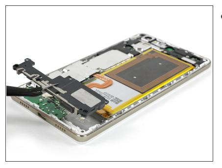
• Remove the loudspeaker carefully.
