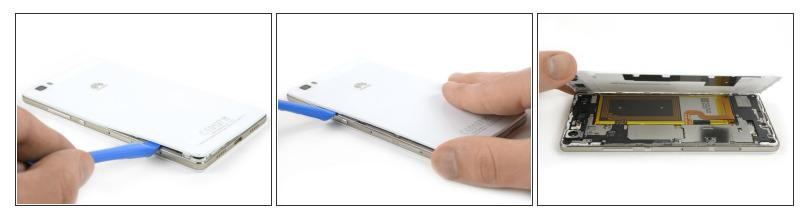
• There are clips around the whole mid frame, holding down the back cover. Open all of them with the Opening Tool.
