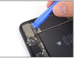
• Use an iFixit opening tool or a fingernail to disconnect the dual camera cable connectors by prying them straight up from their sockets.
