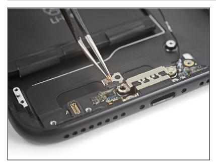
Remove the spring contact underneath the screw you just removed.
