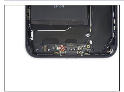
Remove the 2.9 mm Phillips screw at the top left of the Lightning port.
