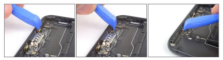
• Use the sharp edge of an iFixit Opening Tool to pry the two microphones free from the adhesive securing them in place.
