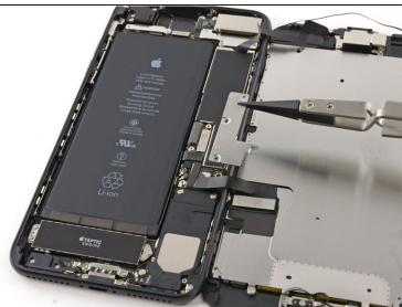
• Remove the lower display cable bracket.
