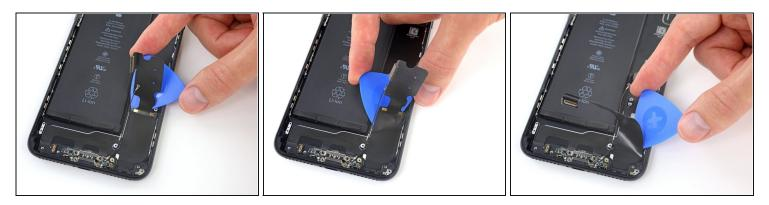
• Continue separating the upper portion of the flex cable, being careful not to damage any other components along the way.
