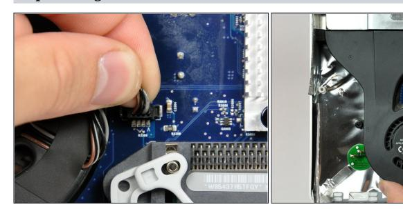
• Disconnect the CPU fan connector from the logic board by pulling it straight up from its socket.
