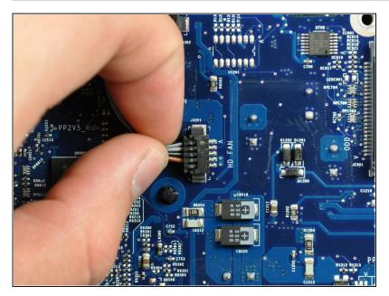
Disconnect the hard drive fan connector from the logic board by pulling it straight away from its socket.
