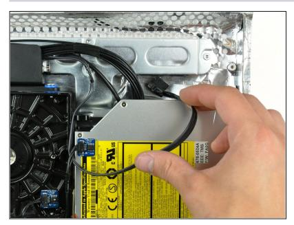
De-route the hard drive data cable and tuck it under the optical drive to prevent the cable from interfering with future steps.
