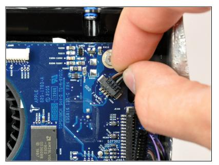
Disconnect the optical drive fan cable connector from the logic board by pulling it straight away from its socket.
