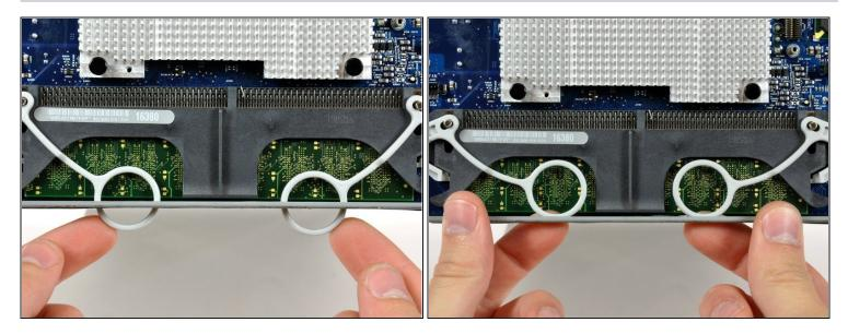
• Push the two RAM arms protruding from the access door inward and set them on the lower edge of the rear case to prevent them from getting caught when removing the logic board.
