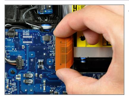
Disconnect the optical drive flex cable from the logic board by pulling it straight up from its socket.
