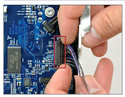
Disconnect the camera board cable connector from the logic board by pulling it straight away from its socket.
