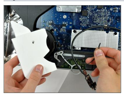
De-route the left speaker cable along its path across the logic board.
