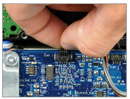
Disconnect the hard drive temperature sensor connector from the logic board by pulling it straight away from its socket.
