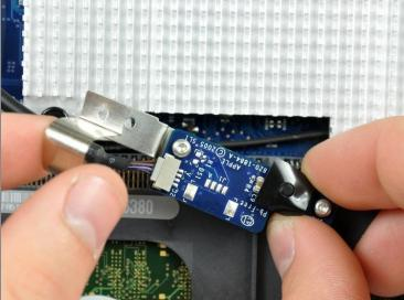
• Remove the single 5 mm T6 Torx screw securing the IR board bracket to the logic board.
