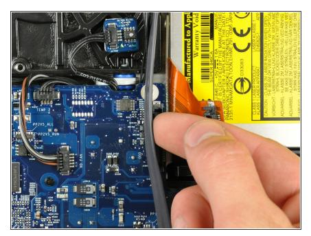
Move the SATA data cable away from the edge of the optical drive.
