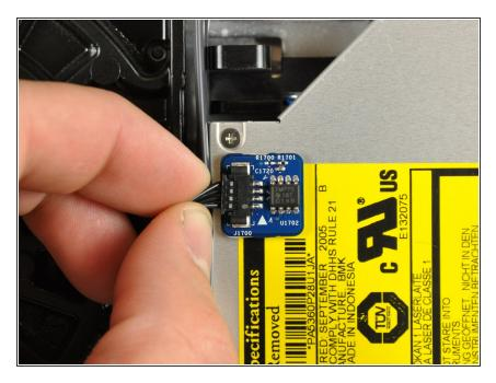
Disconnect the optical drive thermal sensor.
