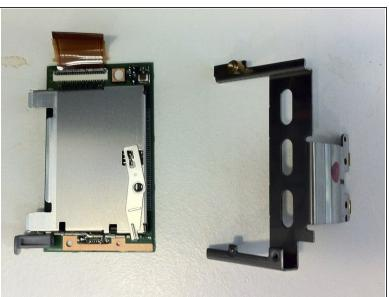
Remove the two Phillips screws to separate the Holder from the Slot.
