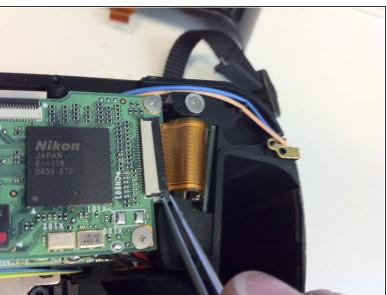
Use Tweezers to open the locking on the ribbon cable socket.
