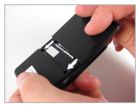
Remove the rear cover by pressing down on the cover and pulling it away from the device.
