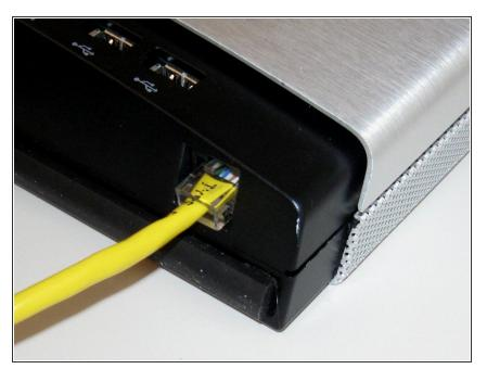
• Connect to the Console Port. Plug the 8P8C (RJ45) end into the console port. You'll have to lean the unit forward to plug the cable in. It might be a little awkward to do alone. If someone else is available, ask for their assistance. As a last resort, lay the unit down. Ensure you have something soft (like a towel) to lay the unit on.
