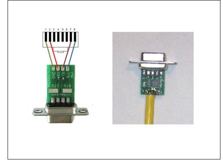
• Connect the RS232 to TTL/CMOS converter. Connect the RS232 to TTL/CMOS converter to the cable and solder the connections. Note: The colors used in the wiring diagram don't correspond to the color of the actual wires.
