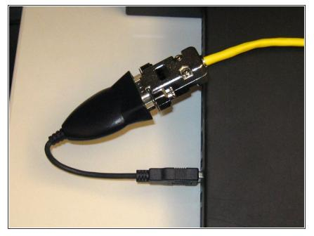
• Connect the DB9 to a USB serial adapter and connect to a laptop/PC.
