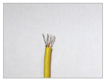
• **Prep the cable.** Strip the sheathing from the wires that correspond to pins 1,2,7 & 8.
