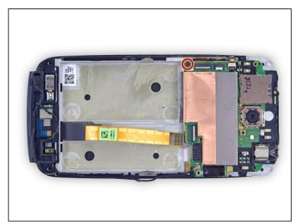
• Remove the 3.15 mm Phillips #00 screw from the motherboard.
