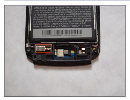
The component denoted in the red box is the vibration motor.
