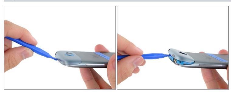
• Starting at the groove near the headphone jack, use a plastic opening tool to lift the top casing.
