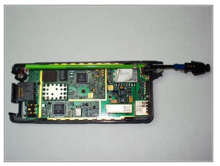
Insert the new antenna into the green tubing.
