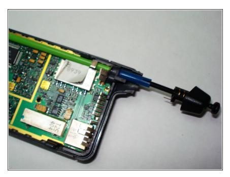
Screw the blue piece of the antenna into the threaded hole on the motherboard until it is tight.
