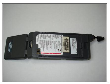
• Reverse the instructions from Step 2 to re-install the keypad guard and rear casing onto the device.
