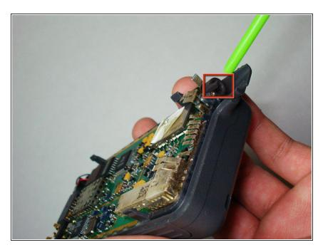
Insert the new green tubing into the corresponding slot.
