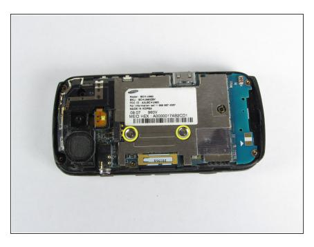
Remove the two 3.45 mm Philips screws below the white sticker.
