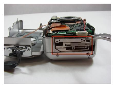
• Use a pair of tweezers and remove the metal piece inside the camera.
