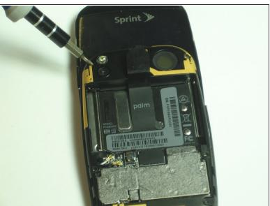
Use the T5 Torx Screwdriver to remove the six screws holding the backing frame in place.
