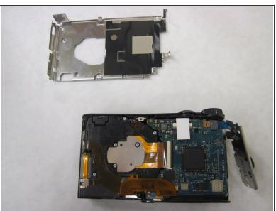
Once the LCD is off use the J00 screwdriver to take out the two 4mm silver screws. Once the screws are taken out pull off the piece with your fingers.
