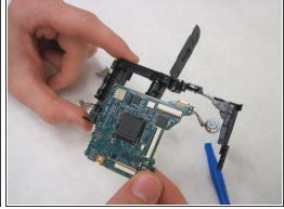
On the backside of the motherboard, a silver clip is holding the motherboard to the plastic shell.
