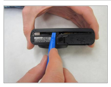
Insert the plastic opening tool between the back cover and the bottom plate. Gently pry the cover off.
