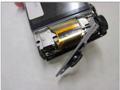
Use your fingers to slide out the controller wheel board.
