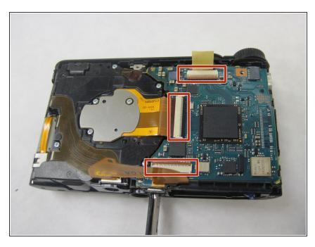
Remove the three ZIFs connected to the motherboard. The top is found under a piece of tape.
