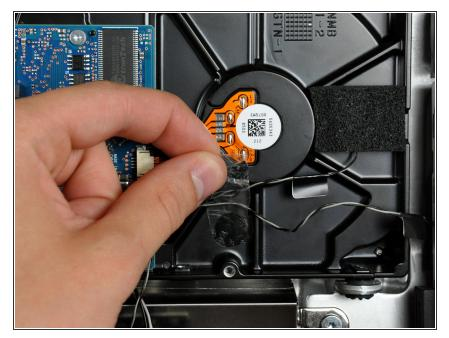
If necessary, remove the piece of tape holding the thermal sensor wires to the hard drive.
