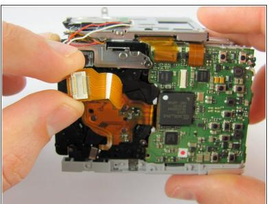
Remove the orange ribbon cable by grabbing the white tab and pulling back.
