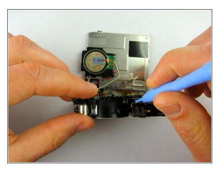
Once the bottom portion of the camera is removed, stand the camera upright, bottom portion facing up, then detach the inner orange strip from the motherboard to the lens by inserting the plastic opening tool under the tab and lifting up.
