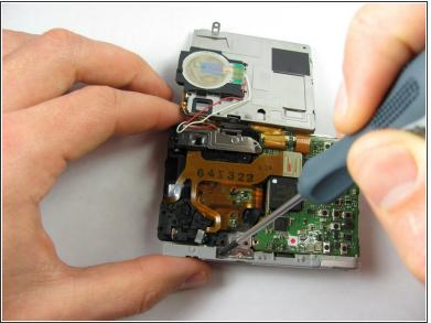
Remove the two 1.66mm screws on both the bottom and top metal plates, using a #00 Phillips screwdriver.
