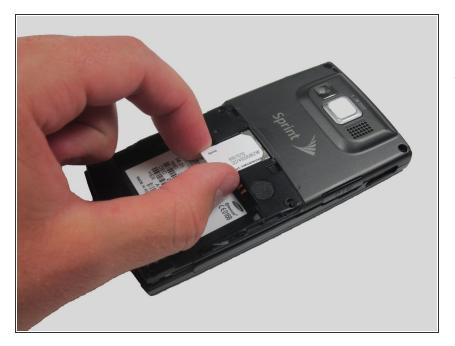
• To remove the SIM card, start by pressing the top of the card and push down and away towards the bottom of the phone. Then, as indicated, pull the SIM card out.
