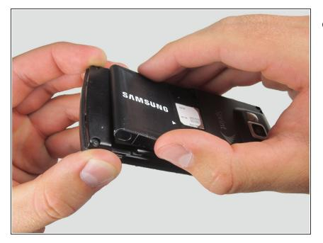
• With the casing removed, lift the battery from the indicated indentation.
