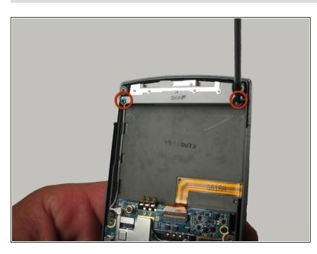
Remove the two indicated screws (3.9 mm) with a Phillips #00 screwdriver.
