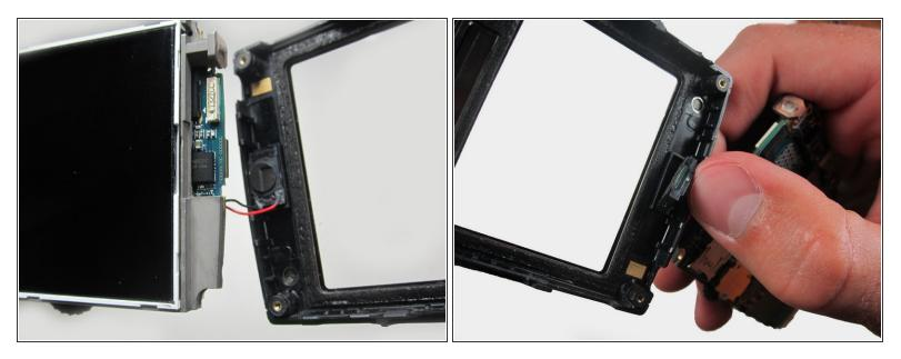
• Gently pull on the wires to remove the front casing.
