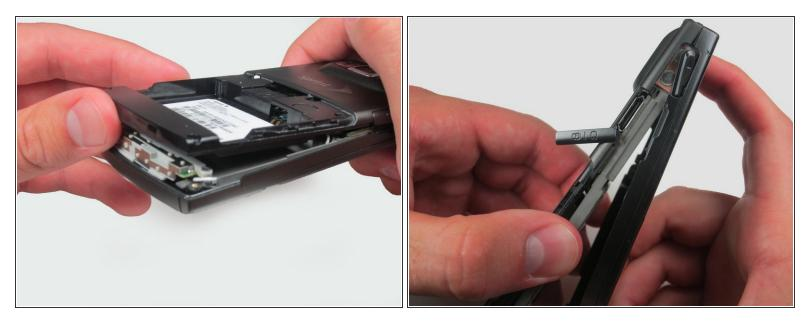
Begin to slowly lift the back casing of the phone. You should hear a snap when the casing is released.
