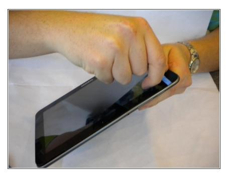
Insert a plastic opening tool between the back cover and screen of the Samsung Galaxy Tab 8.9 (as indicated in the photograph).
