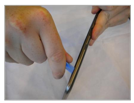
Slide the second plastic opening tool along the edge of the device to separate the back cover.
