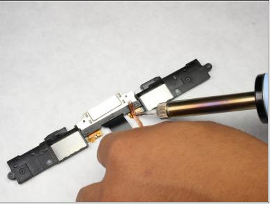
Desolder the two connections to separate the speakers from the charger port.
