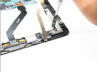
Using a Phillips #00 screwdriver, unscrew the 4 screws (3mm) that are holding the charger port and speaker support.
