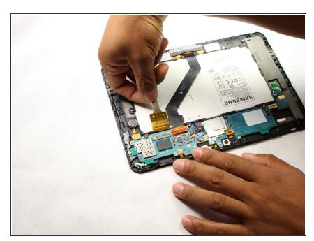
Slide out the yellow flexible ribbon cable to disconnect it from the motherboard.
