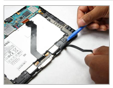
Insert opening tool to pry support from the housing.
