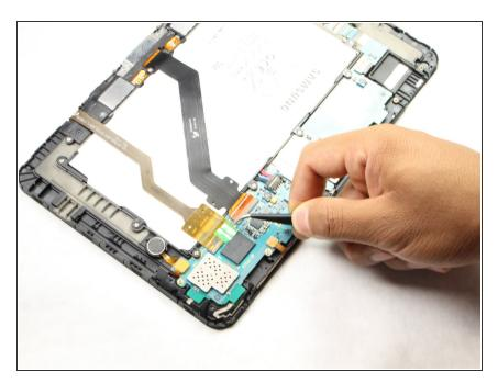
Using tweezers, peel away the green tape located on top of the two flexible ribbon cables.
