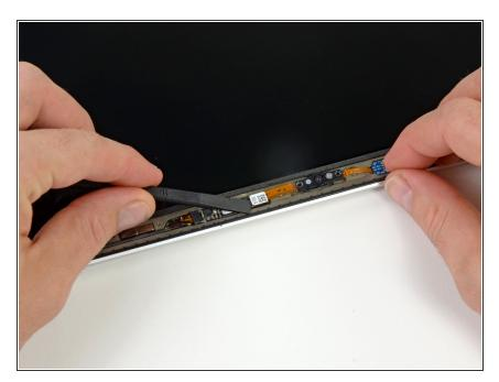
Use the flat end of a spudger to pry the iSight cable connector off its socket on the camera board.
