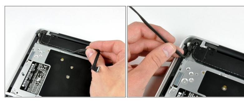
De-route the camera data cable from the channel in the optical drive.
