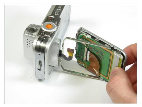
• Pull the screen away from the camera the same way that you removed the screen backing.
