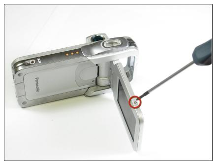
Remove the screw(2.6mm Philips) indicated on the top of the screen with the screwdriver. Then remove the corresponding screw on the bottom of the screen.
