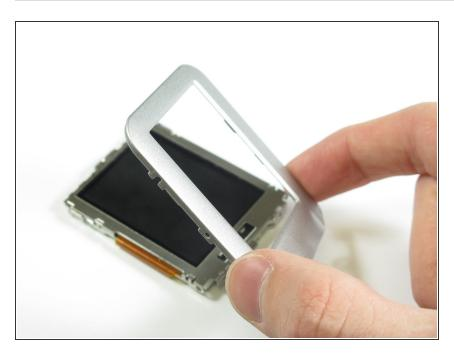
• Pull upwards on the screen border to remove it from the actual screen.
