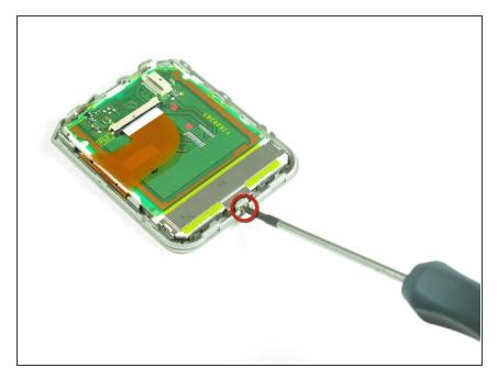
• Use the screwdriver to remove the screw(2.46mm Philips) indicated.
