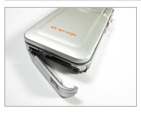
Pull/lift open the battery cover in the direction directly away from the camera.
