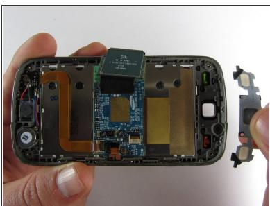
In this procedure, the rubber function key pad can easily fall out, so it would be best to take it out and set it safely aside.
