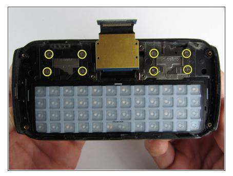
Remove the eight 1.7mm Philips screws above the keyboard.
