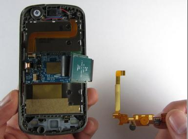
Using tweezers, gently remove the bottom orange strip from the device
