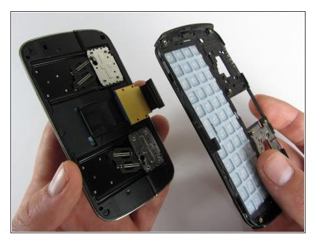
Carefully remove the keyboard frame from the sliding mechanisms underneath.
