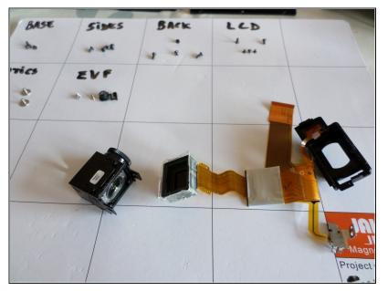
Adhesive sealing tape can be just worked out with tweezers to unstick it without removing it.
