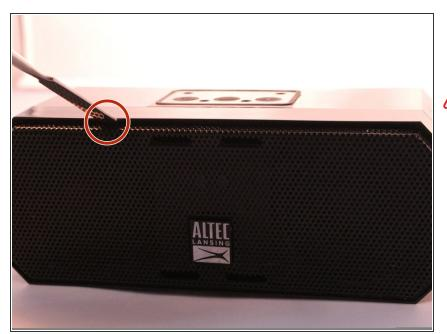
• Pull out the two black wire meshes using a metal spudger.
