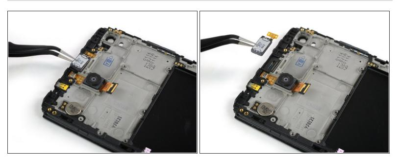
Use a pair of tweezers to carefully lift the earpiece speaker out of the device and remove it.
