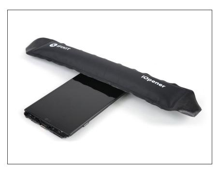
Use an iOpener to loosen the adhesive beneath the earpiece speaker and its flex cable.
