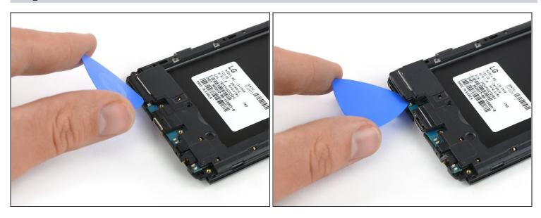
• The loudspeaker is attached to the cover of the motherboard. Use an opening pick to pry it up.
