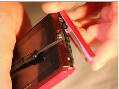
Pull the edge-casing off of the camera.
