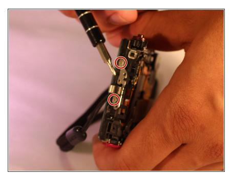
Using a Phillips #00 screwdriver, remove two silver 3mm screws from the side of the device.
