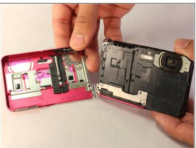
Remove the front casing of the device.
