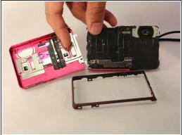
Using the plastic opening tool, remove the back casing of the device.
