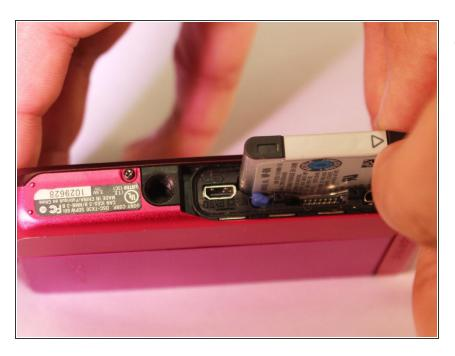
Remove the battery from the device.
