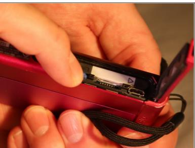
Push the battery eject lever to free the battery.
