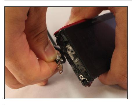
Using your fingers, remove the silver wrist band holster from the device.
