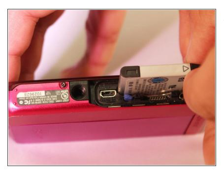
• Remove the battery from the device.
