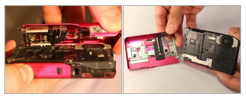
• Remove the front casing of the device.
