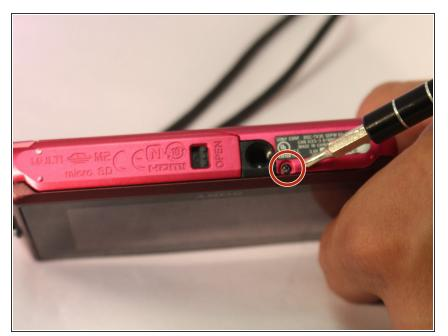
Using a Phillips #00 screwdriver remove one black 2 2/5mm screw near the tripod slot on the bottom of the casing.
