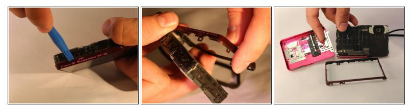
• Using the plastic opening tool, remove the back casing of the device.
