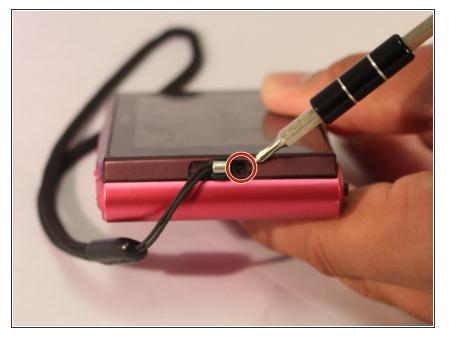
Using a Phillips #00 screwdriver, remove one black 2 2/5mm screw that is located next to the wrist band loop.
