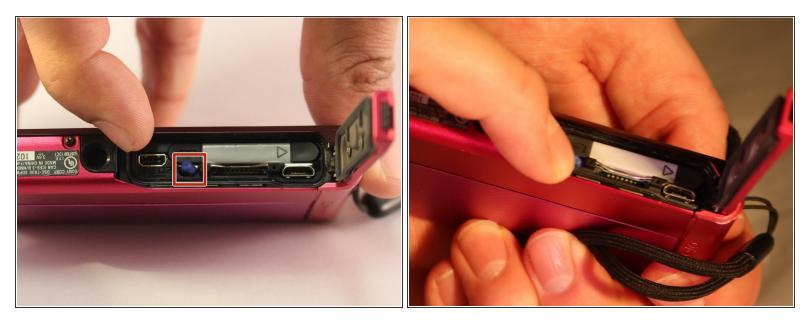
• Push the battery eject lever to free the battery.
