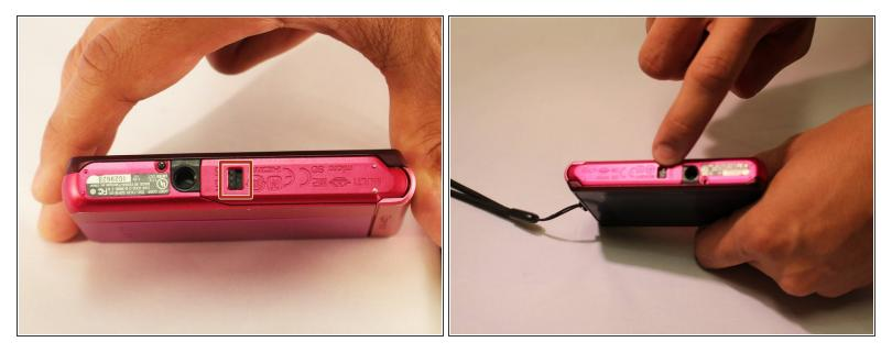
• Using your finger, slide the release catch to unlock the battery/memory card cover.
