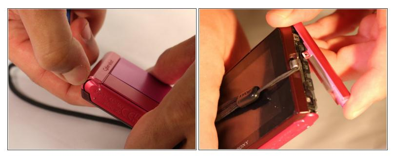
Pull the edge-casing off of the camera.
