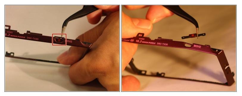
• Using the tweezers, remove the movie button from the back casing of the device.
