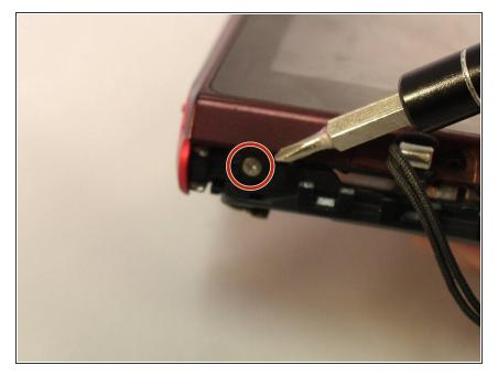
Using a Phillips #00 screwdriver, remove one 2 1/2mm screw located near the wrist strap.
