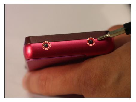
Using a Phillips #00 screwdriver remove the two 2 2/5mm black screws from the side of the camera opposite of the wrist strap
