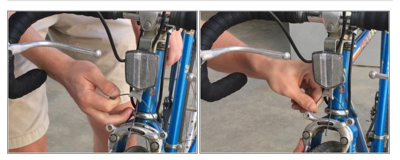
Reattach the brake cables to the brifters and brake calipers
