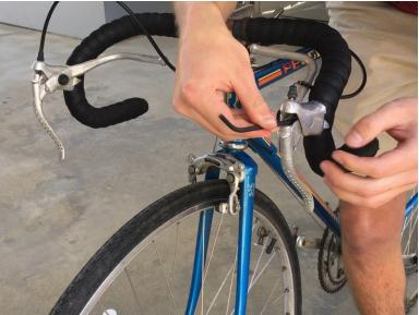
Using the 5mm Allen key, reattach and tighten the brifter levers onto the handlebar.
