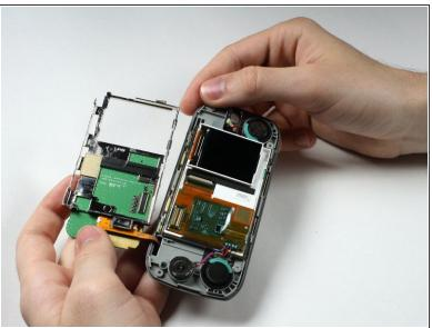
Because the Number Keypad is attached on one side and on top of the outer screen, open its metal casing, in a "door-opening" manner.
