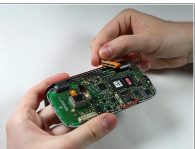
Gently pry and detach the connection located near the hinge with fingers.
