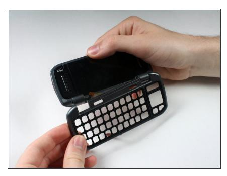
After removing the circuit board and key board, separate the top part with the screen from the bottom part by detaching the hinges.
