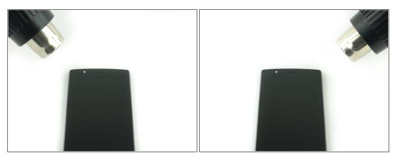
• Use a heat gun or an iOpener to soften the adhesive underneath the edges of the screen.
