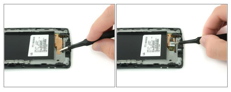
• Use a pair of <u>tweezers</u> to remove the adhesive strip that secures the digitizer ribbon cable.
