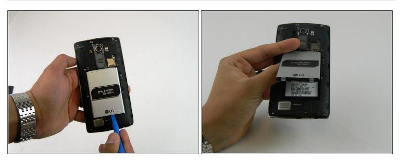
Place the plastic opening tool at the bottom edge of the battery and lift up. Carefully remove battery with your hands.
