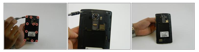
Remove the **eleven** 3.9 mm Phillips #00 screws found at the back of the phone.
