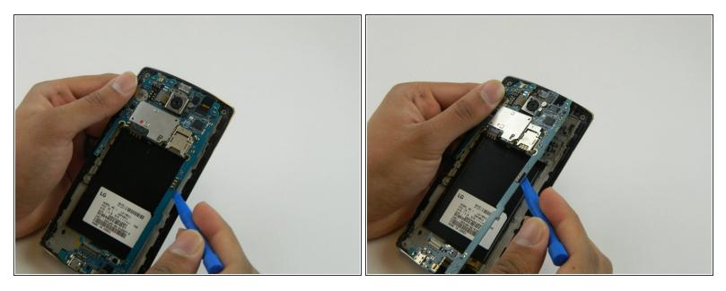
Remove the motherboard by lifting it up using the plastic opening tool and your fingers.
