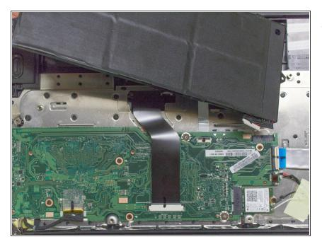
• Carefully lift the entire battery pack out of the laptop.
