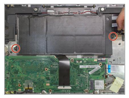
Remove the two 4mm Phillips #0 screws on either side of the battery pack that are securing it in place.
