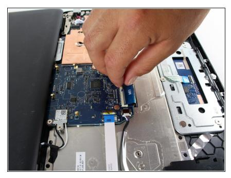
Disconnect the ribbon cable from the motherboard. To do this, lift up the black tab hinge securing the ribbon cable and pull the cable up and then out of the port.
