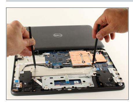
Release the keyboard from the body. To do this, push on the two keyboard release holes with something thin and cylindrical like a spudger or a pencil.
