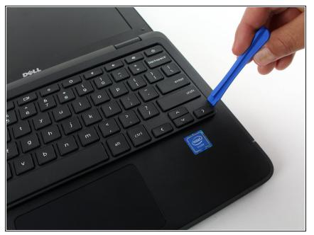
Remove the keyboard from the body. To do this, use a plastic prying tool to get under the keyboard and pry it up from the computer body.
