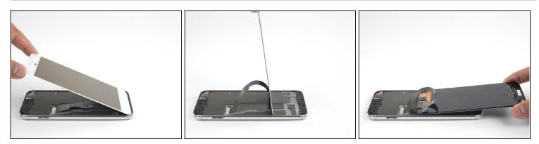
• Lift the display assembly from the top end and swing it around such that it rests upside down on the frame.
