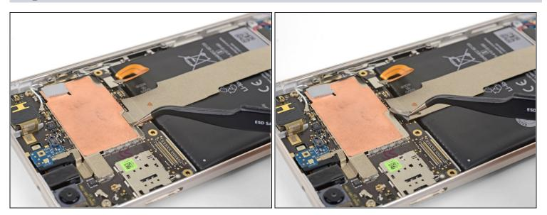
• Use <u>tweezers</u> to peel up the tape at the top of the interconnect cable.
