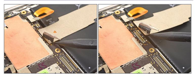
• Use the point of a spudger to pry up and disconnect the interconnect cable from the motherboard.
