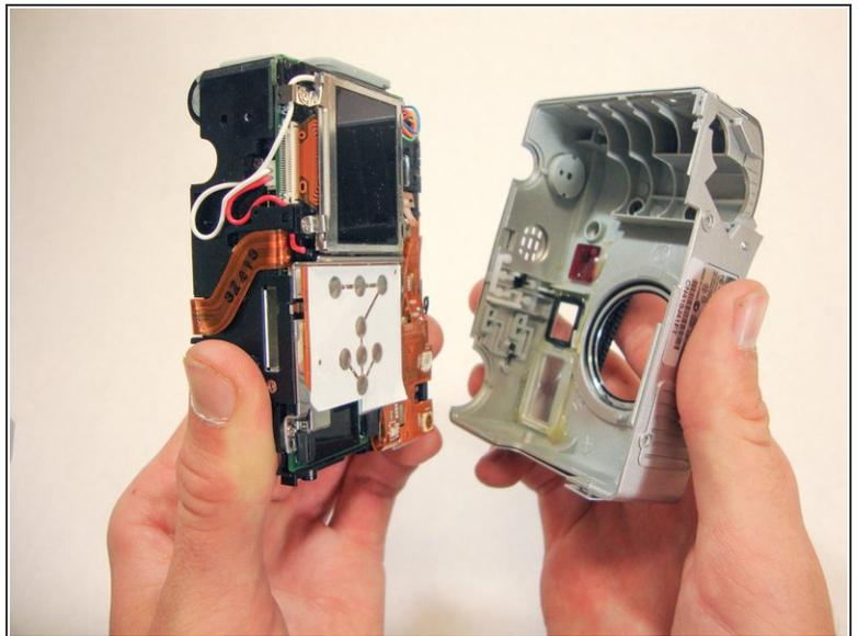
**⚠** While pulling the camera out of the case, note the small soft plastic cover on the side. This cover will detach from the rest of the device.
