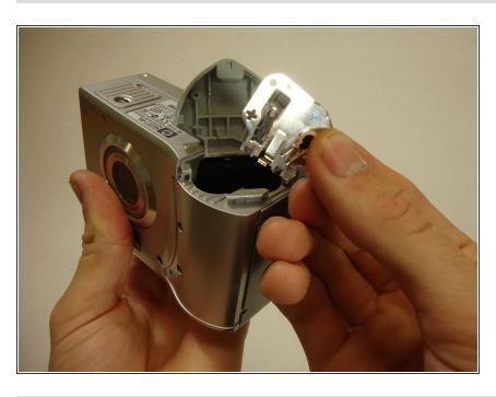
Remove the connector from the battery holder door.
