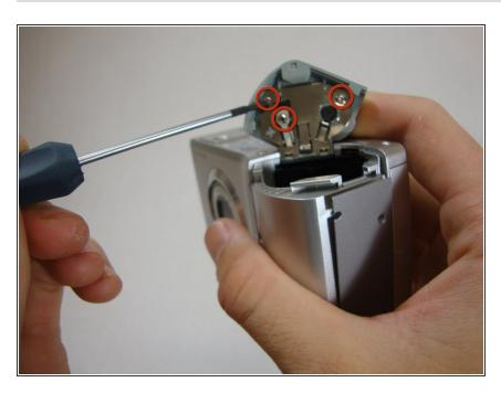
Remove the three screws from the circuit connector.
