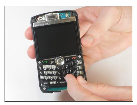
Lift the flexible keypad away from the device. It should come off easily.
