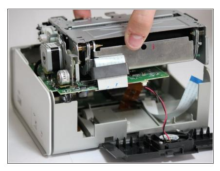
Carefully remove the inner components of the device by lifting the inner components up and out of the casing.
