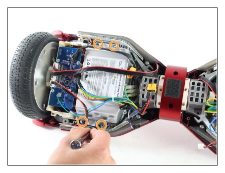
Unscrew the four 9.4 mm Phillips #1 machine screws attaching the battery to the base of the Swagtron T3.
