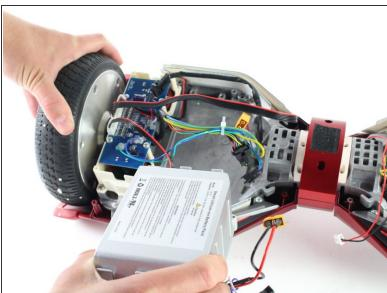
Remove the battery by pulling it out from under the cables.
