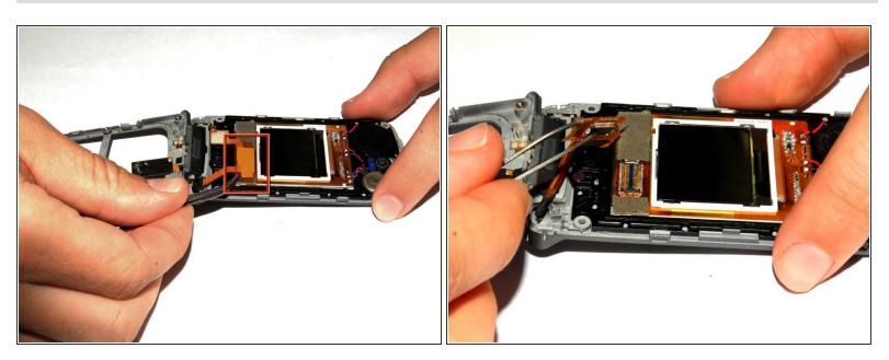
Use the tweezers to lift the display adapter off the screen component.
