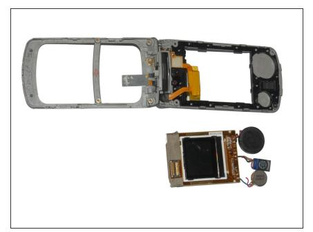
Lift the screen components out of the phone.
