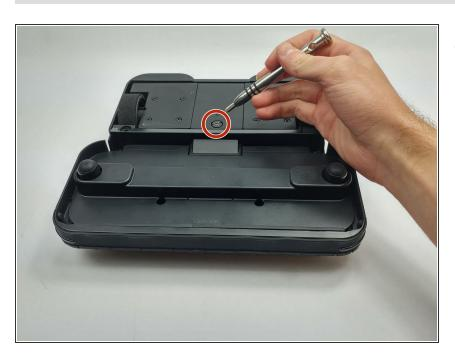
Using a 4mm flat head screw driver, remove the screw holding the battery cover.
