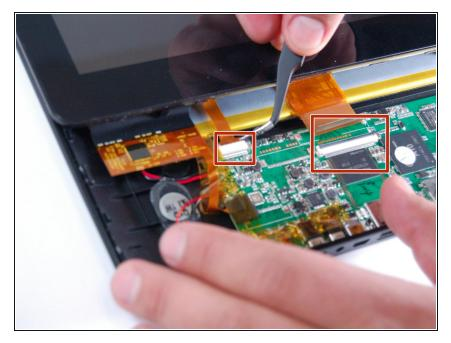
Use a spudger to carefully disconnect the display ribbons from the motherboard.
