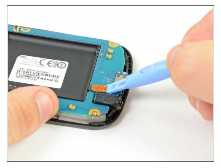
Insert the flat edge of a plastic opening tool underneath the headphone jack connector and pry upwards.
