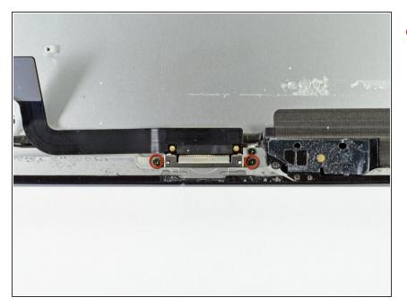
Remove the two 1.8 mm Phillips #00 screws securing the dock connector to the rear aluminum case.
