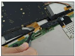
• Begin by removing the ribbon on the right. With the curved <u>tweezers</u>, carefully remove the metal bracket to expose the end of the ribbon. Remove ribbon.
