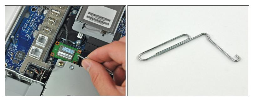
Bend a paper clip into a hook and use it to pull the Bluetooth board up off its socket on the logic board.
